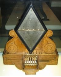
Cooke and Wheatstone telegraph, 1837. The five needles were controlled by six wires, and the intersection of the needles that moved indicated the letter. Source Wikipedia Commons ( https://en.wikipedia.org/wiki/Telegraphy#/media/File:Cooke_and_Wheatstone_electric_telegraph.jpg )
