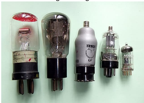
The evolution of triode vacuum tubes from a 1916 model (left) to one from the 1960s. (Image courtesy of Wikipedia user RJB1.)
