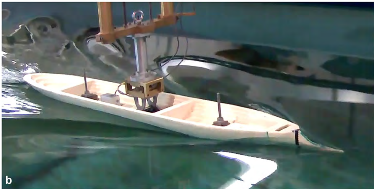
a) Control bow showing wave build-up at 10 knot equivalent; b) cutwater bow showing wave attenuation at 11 knot equivalent.
