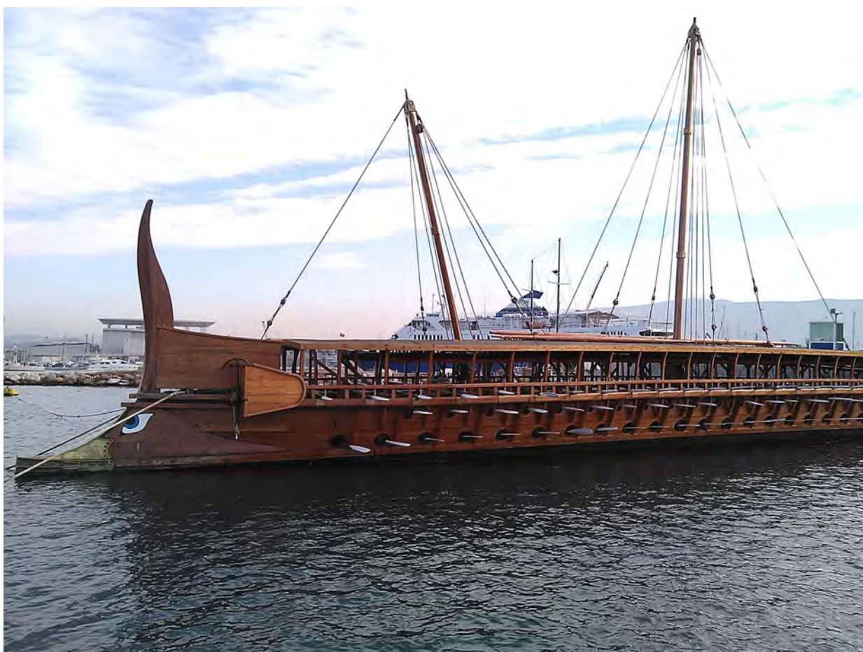
Olympias showing her bow, with bronze ram and sides of the ship.
