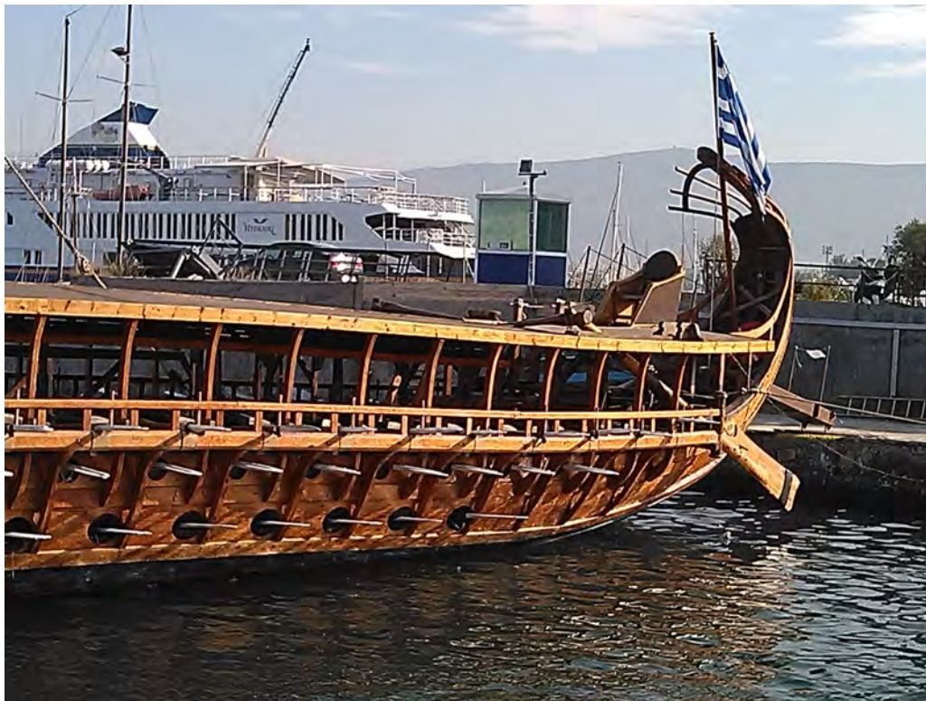
Stern detail showing the seat for the trierarch (captain) who sat directly behind the two kybernetoi (steersmen) who handled the steering oars.
