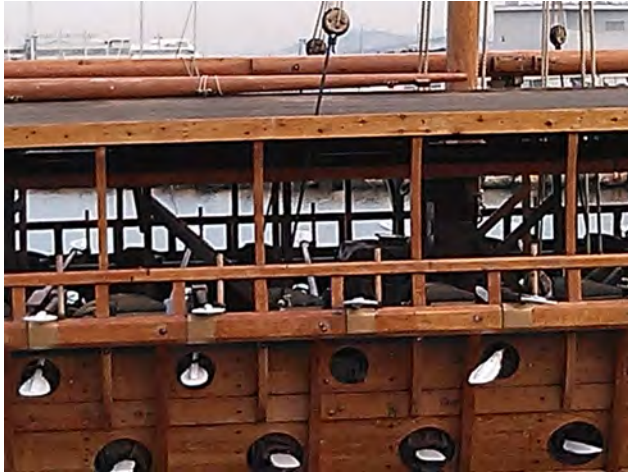
Athena's "wooden walls": midships detail of Olympias showing her oars retracted and the mainmast footings.
