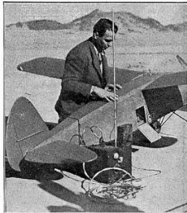
Paul Whittier, chief engineer of Reg Denny's radio-control model venture, is checking the details before the $2,100 job is sent "upstairs." That opening in the fuselage leads to the chamber for the receiving unit. No ailerons are used on this ship, entire control being achieved through the rudder and elevators.
